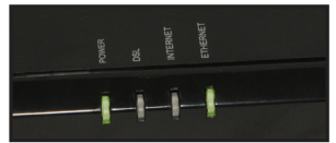
NOTE: IF THE ETHERNET LIGHT DOES NOT TURN GREEN, MAKE SURE THE YELLOW CABLE IS PROPERLY CONNECTED ON BOTH ENDS.
